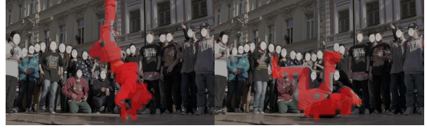
Figure 9. Motion-Aware Representations. We cluster PCA-reduced intermediate image tokens by k -means and observe that the resulting clusters consistently separate the moving dancer from the static crowd and background, with red indicating high-response regions. This suggests that VGGT- \Omega learns motion-aware representations from reconstruction training, without explicit motion supervision.
